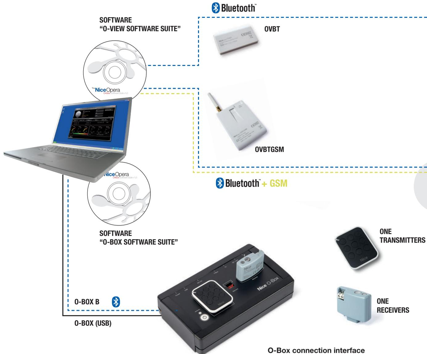
**O-Box connection interface** which, thanks to the "O-Box Software Suite", enables the configuration and programming of all Nice control devices, from the PC or PDA.
