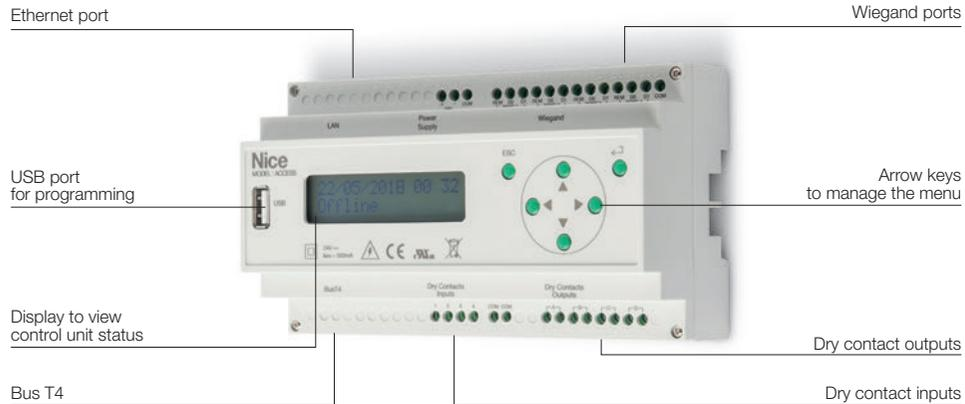
**DIN module for access control with BusT4 output, 4 Wiegand ports, 4 dry contact inputs used as input contacts and 4 used as output contacts, ethernet port.**
