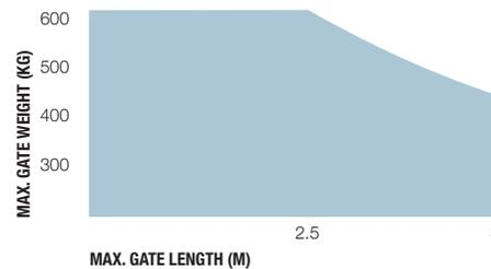
The shape, the height of the gate and the weather conditions can considerably reduce the values shown in the graph to the side. Use in windy areas 230 Vac models.
