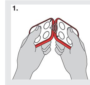
1. Code exchange between a memorized transmitter and a new one, to be memorized.
