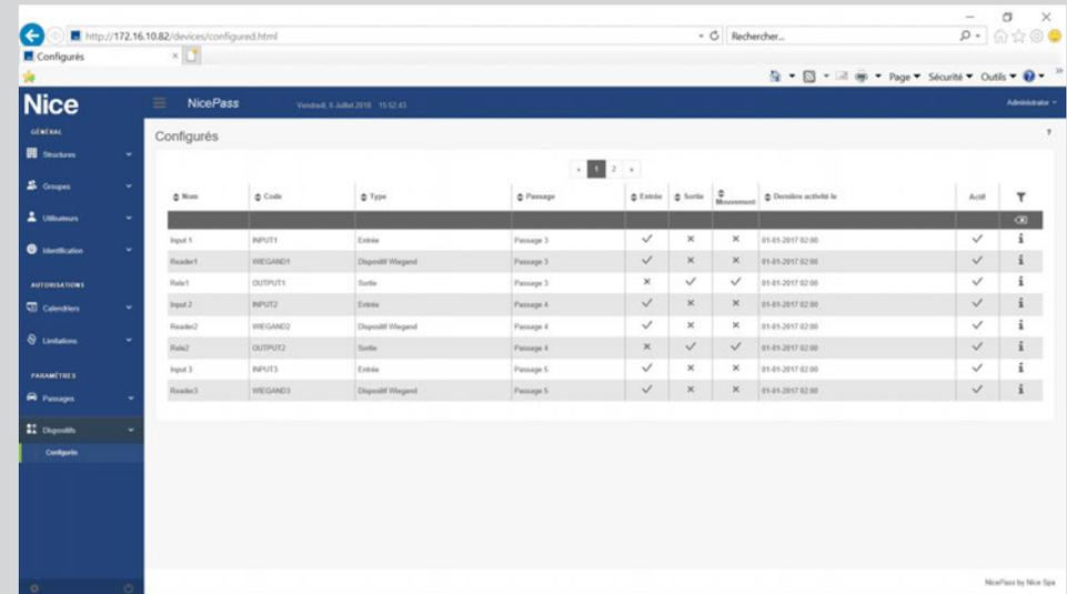
3. The administrator can configure the system architecture completely, by simply selecting inputs and outputs, combining devices and creating areas.
