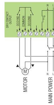
Connections for 2 independent switch outputs
