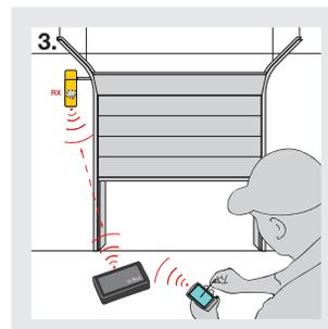
The presence of a "transmitter" in the OXIT, OX2T and OX4T receivers allows radio codes to be accessed by means of the O-Box multifunction interface.
