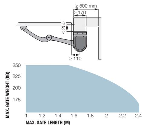
The shape, the height of the gate and the weather conditions can considerably reduce the values shown in the graph to the side.
