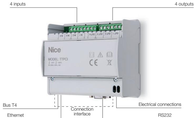
**The TTPCI electronic device allows Nice products to be interfaced with other automation systems and controlled by PC.**
