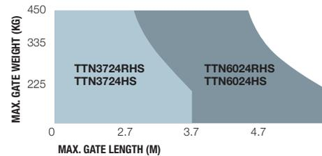
The shape, the height of the gate and the weather conditions can considerably reduce the values shown in the graph to the side.
