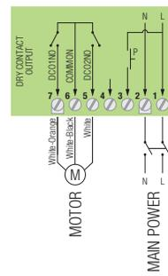
Connections for 3-wire mechanical motor outputs
