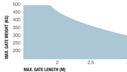
The shape, the height of the gate and the weather conditions can considerably reduce the values shown in the graph to the side.
