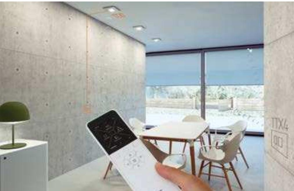
Miniaturised control units and universal concealed transmitters for practical radio management of rolling shutters, awnings, blinds, lighting and electrical loads up to 500 W not reachable directly by cable.
