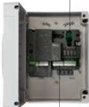
Removable terminals screen-printed with indication of connection
