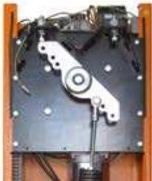
**Balancing springs** - highly robust, guaranteed for up to 2,000,000 manoeuvres for M-Bar and L-Bar models.
