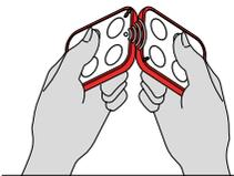
**Exchange of identity code** between a previously memorised transmitter and a new transmitter to be memorised.
