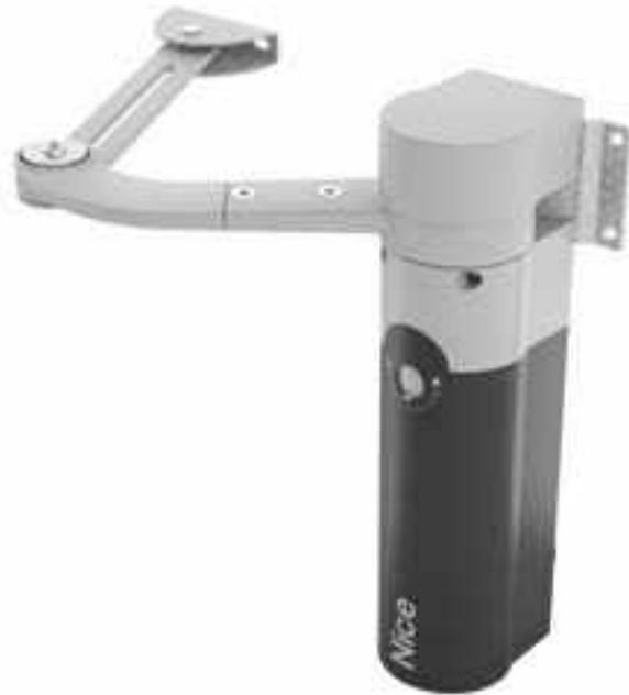
Electromechanical gearmotor, non-reversible, 24 VDC, with articulated arm.
