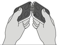
**Exchange of identity code** between a previously memorised transmitter and a new transmitter to be memorised.
